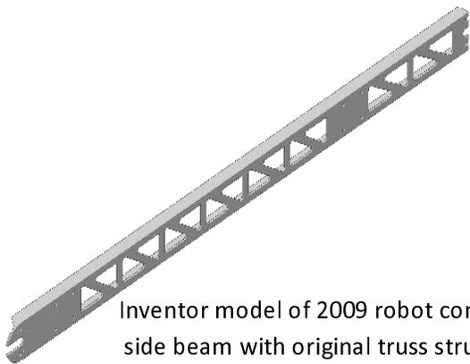
Inventor model of 2009 robot conveyor side beam with original truss structure
