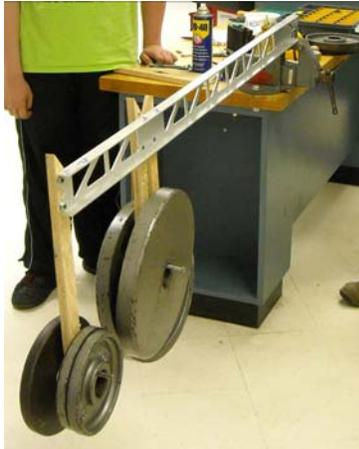
We bolted and clamped the original and new lightened truss to the side of a bench and gradually added free weights.
