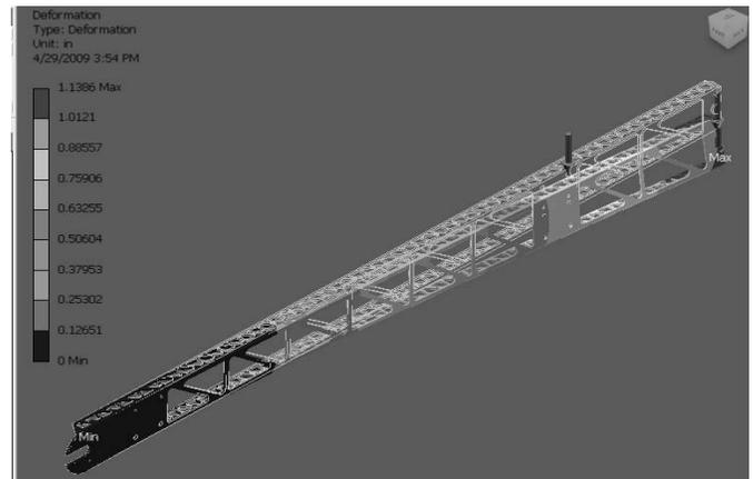
Inventor Stress Analysis predicted a 1.125" deformation with 75 lb load. Actual test resulted in 1.25" of deformation.
