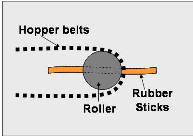
Figure 3. Rubber sticks used to eject balls from the hopper
